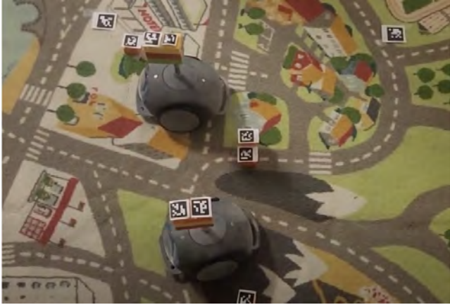
Figure 6: Objects in the physical playground are assigned unique ArUco Codes to detect their type and keep track of their movement.
